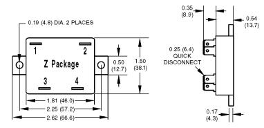
NOTE: All dimensions are nominal. We do not recommend mounting the terminal side of the SSR to a flat PCB (printed circuit board) or other flat surface, because there may be some variation in terminal height or alignment from one terminal to another and from one SSR to another.
