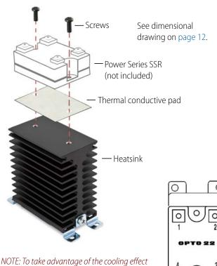
of natural air flow, mount the SSR/heatsink assembly to a vertical surface with the Opto 22 logo right side up as shown here.
