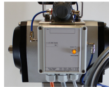
Seal Control Box With power supply and LED indicator
